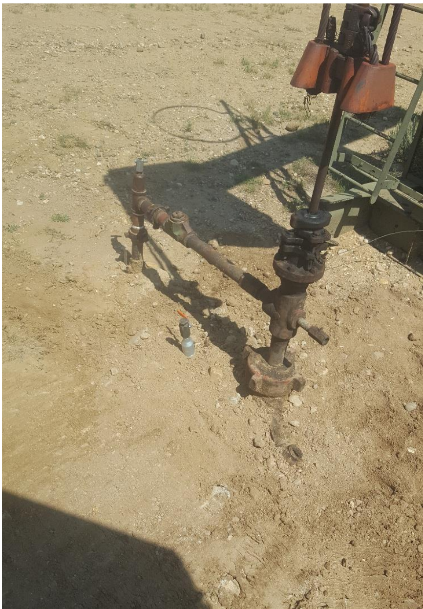
Figure #1 Bradenhead access has been installed.
