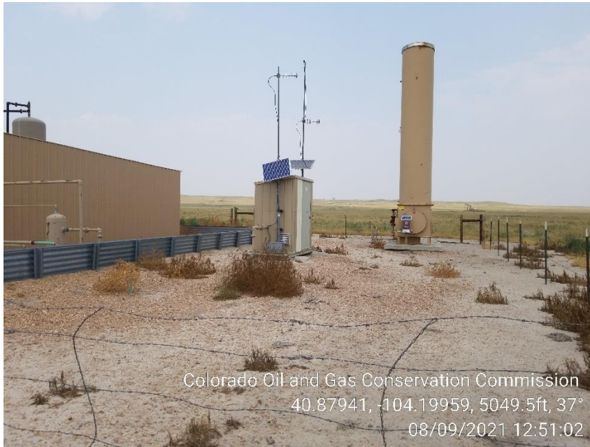
Photo 3 – Gas Meter and ECD
