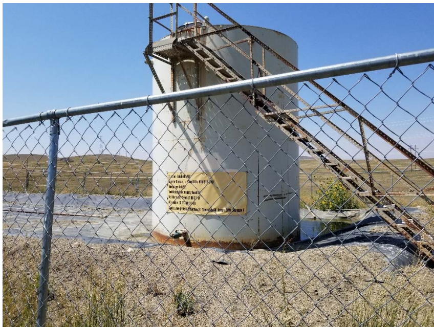
Photo 4. Tank battery banner (sign) on tank. No tank label.
