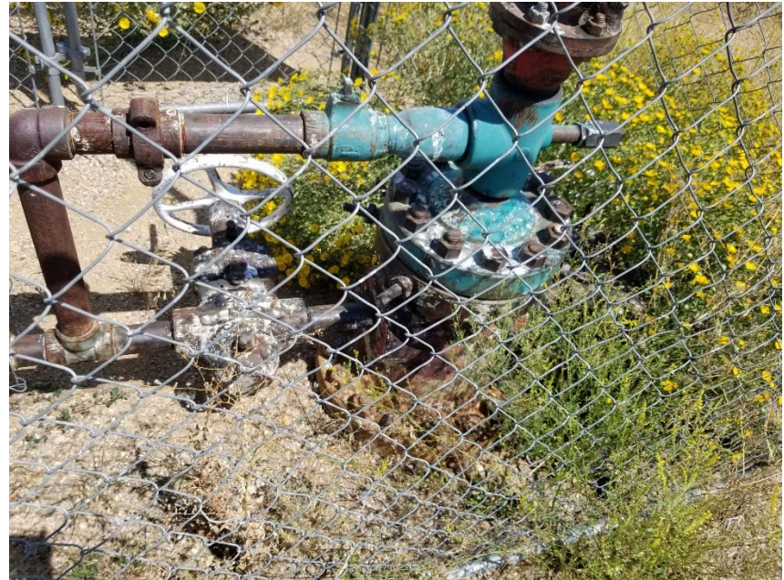
Photo 3. No bradenhead access apparent.
