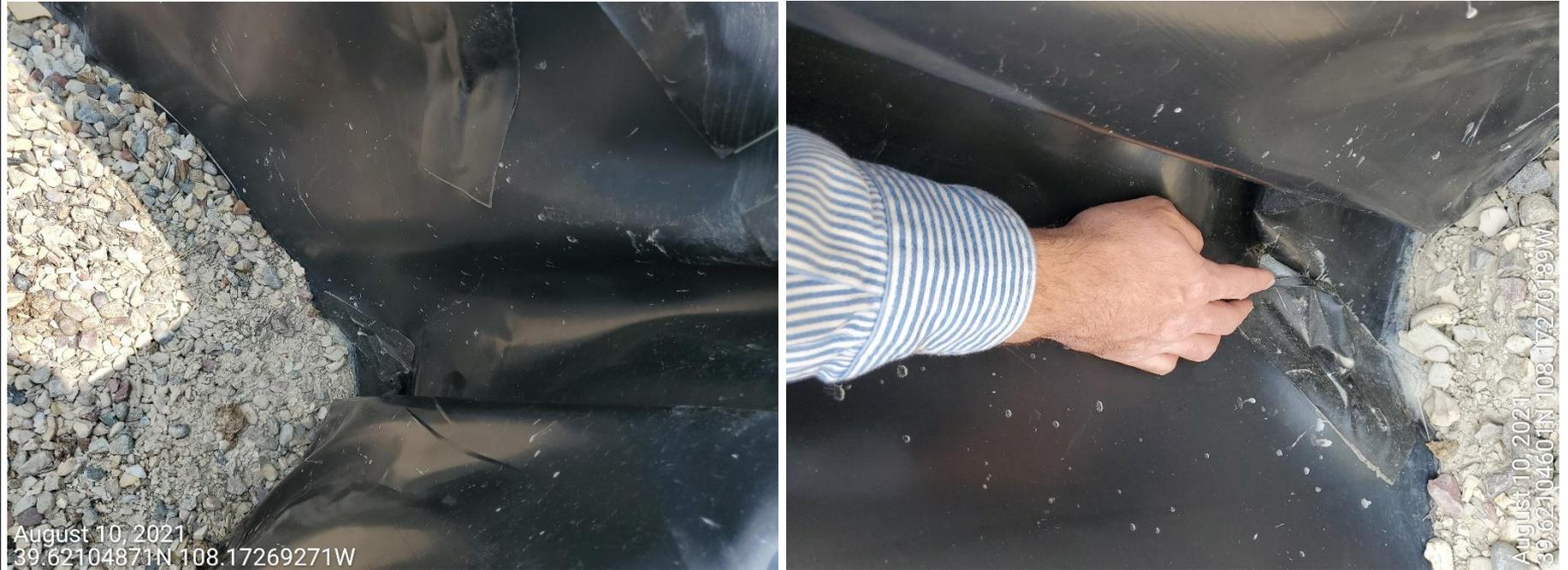
**Photo 1:** Photo patches are peeling away from the secondary containment liner.
