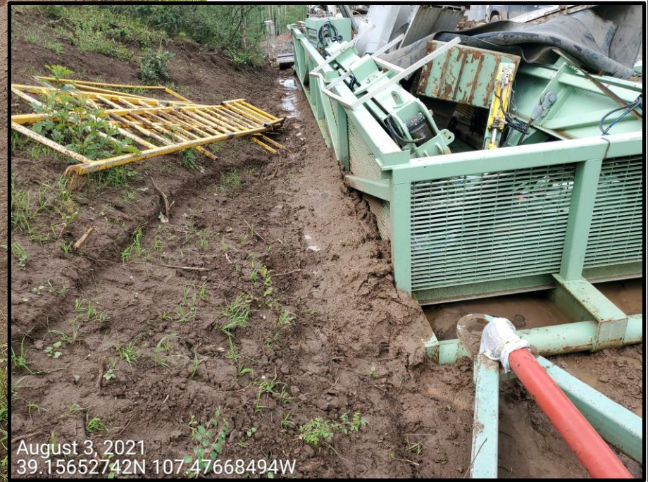
Photo 8: Photo shows equipment remains improperly stored/placed within the stormwater diversion ditch on the eastern and southern perimeter of the pad.
