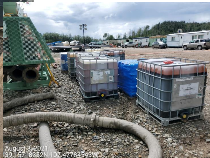
Photo 16: Photo shows example of barrels/tanks/containers observed stored on the Location without proper secondary containment. This issue was documented in the previous inspection; BMPs remain missing or insufficient to contain a spill.
