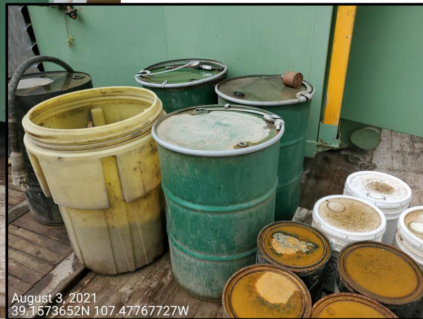
Photo 15: Photo shows green barrels with unknown contents; photo shows example of barrels, and containers where labeling information remains missing. This issue was documented in the previous inspection.
