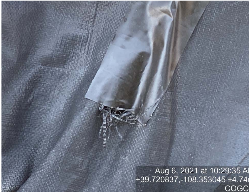
Hole in containment
