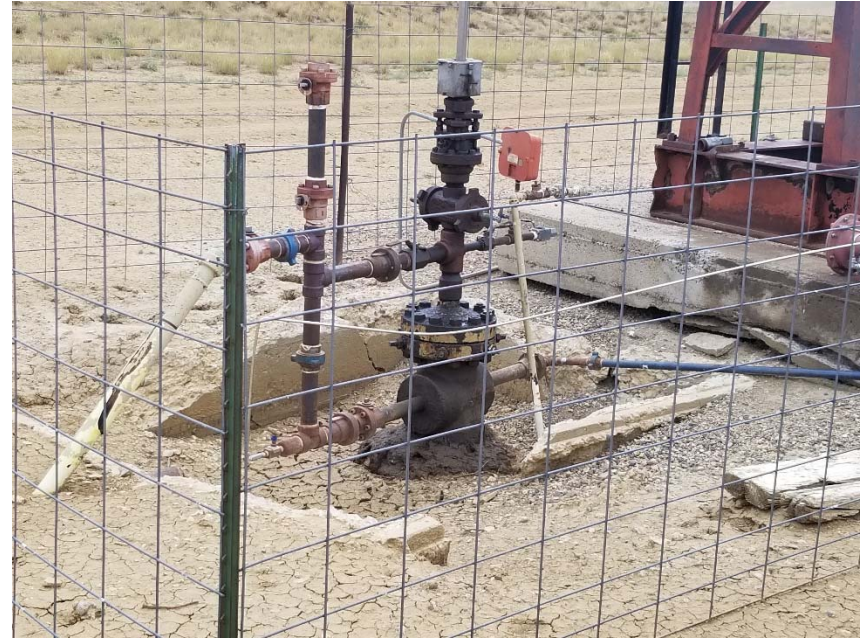
Photo 2. No bradenhead access apparent.
