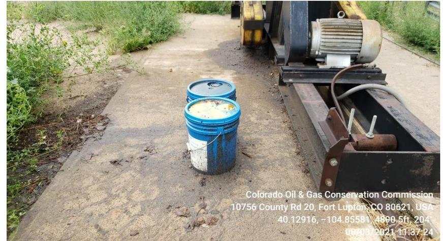
**Photo 7 stained concrete pad under pump jack**
