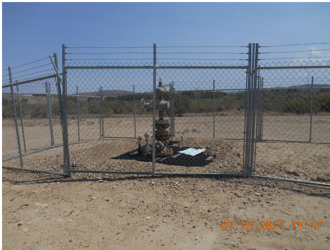
Injection Wellhead – Temporarily Abandoned
