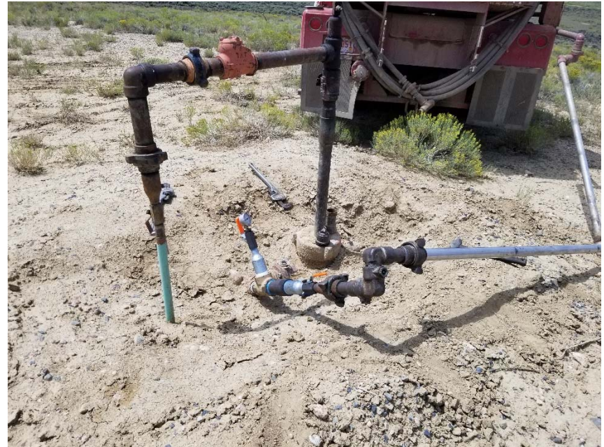
Photo 2. No bradenhead access apparent.
