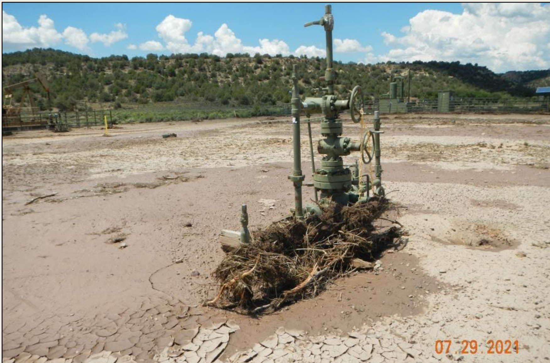
Photo 13. View of woody debris around wellhead.
