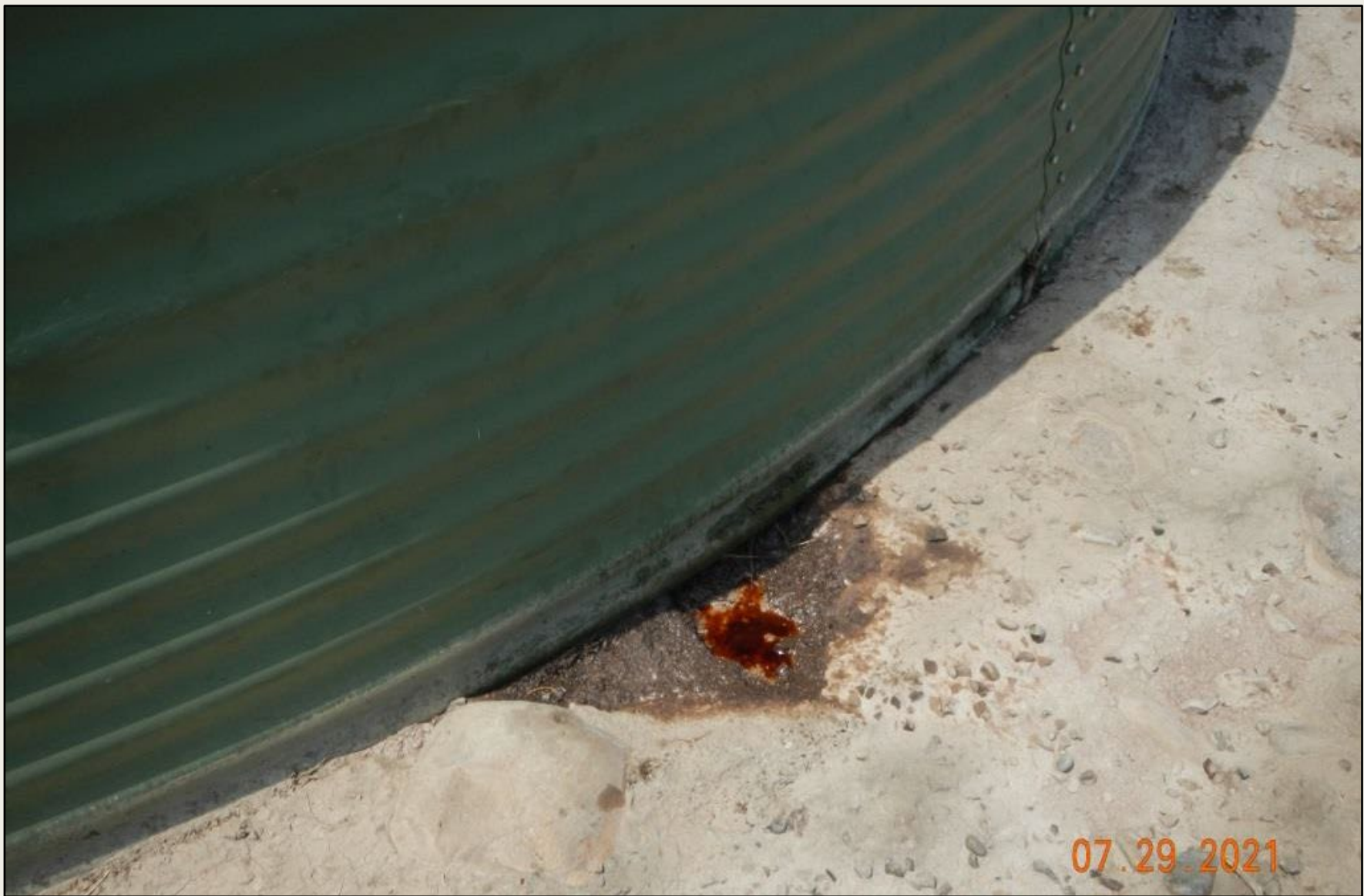
Photo 12. View of pooled material outside of tank containment.
