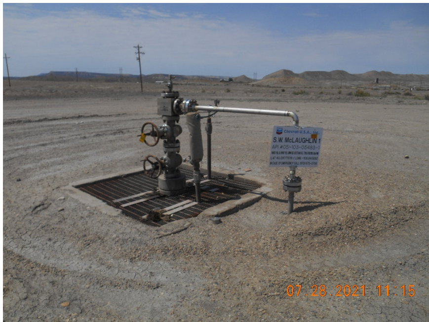
Injection wellhead
