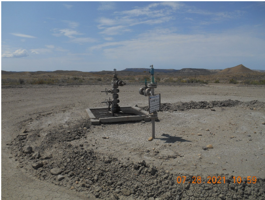
Injection wellhead. Temporarily abandoned.
