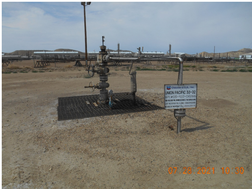
Injection wellhead.
