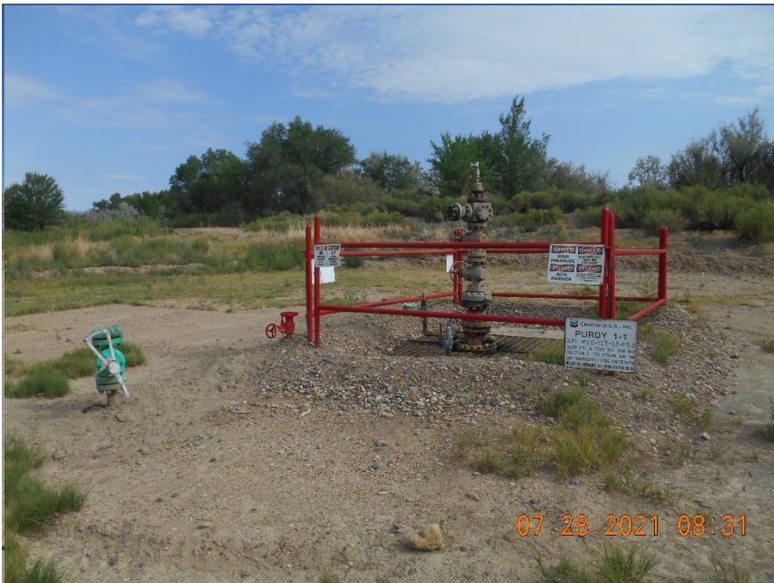
Injection wellhead. Temporarily Abandoned.
