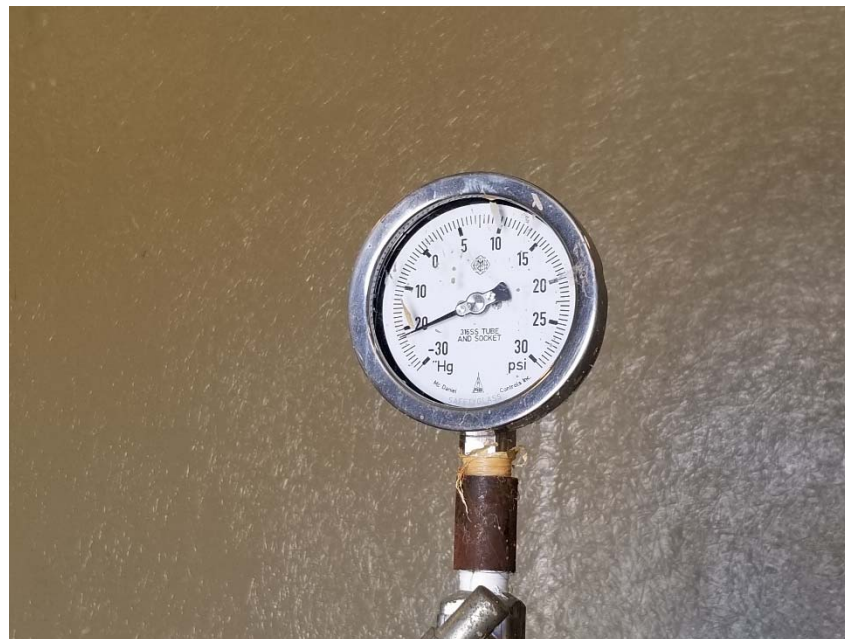
Photo 3. -20 psi vacuum on shut in well.
