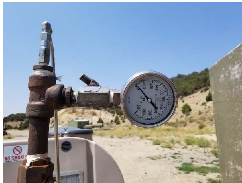
Photo 3. Well shut in at time of inspection.
