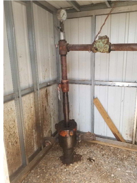
Photo 2. No bradenhead access apparent.
