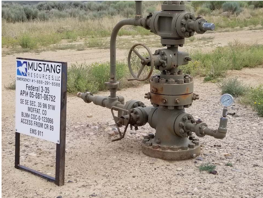
Photo 2. Sign not updated to reflect current operator. No bradenhead access apparent.
