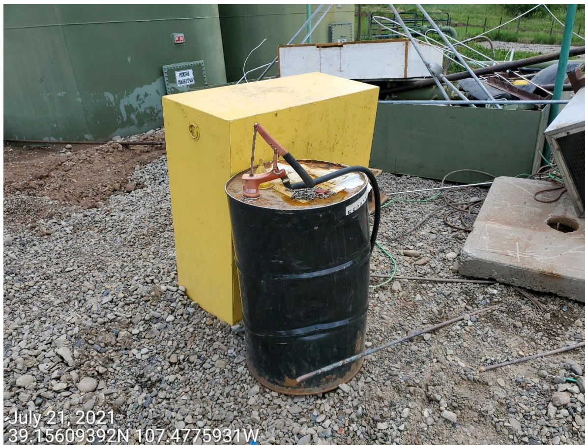
Photo 7: Photo shows barrel containing antifreeze/coolant. Barrel requires secondary containment.
