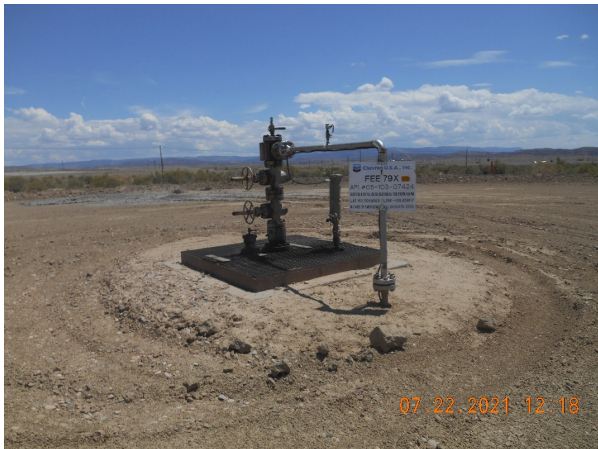
Injection wellhead
