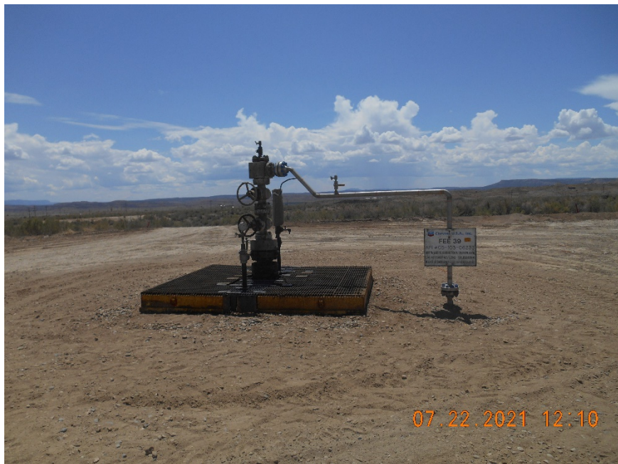
Injection wellhead
