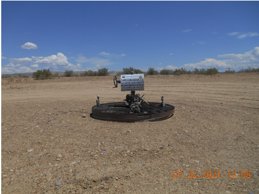
Injection wellhead. Temporarily Abandoned.
