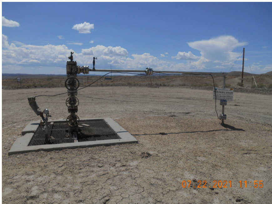
Injection wellhead
