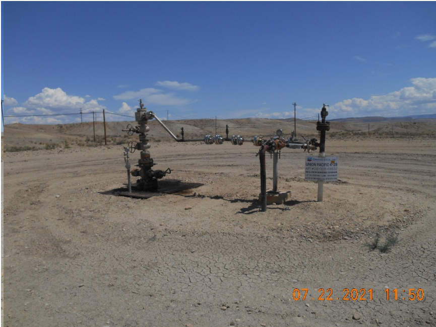
Injection wellhead
