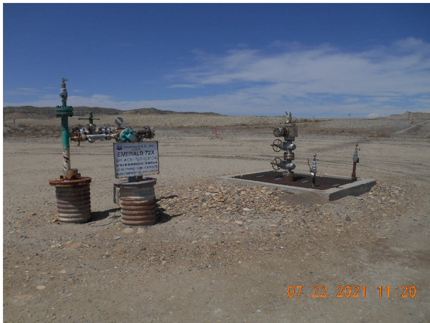
Injection wellhead. Temporarily Abandoned.
