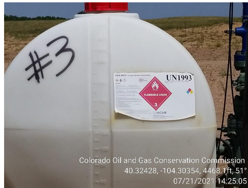
Photo 6 – Label Installed – Starting to Peel
