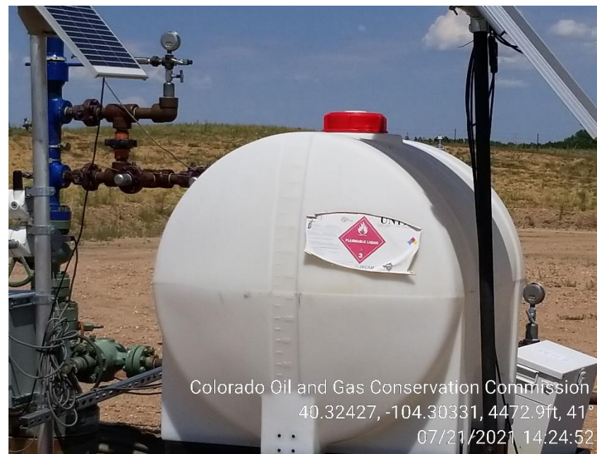
Photo 4 – Label Installed – Starting to Peel
