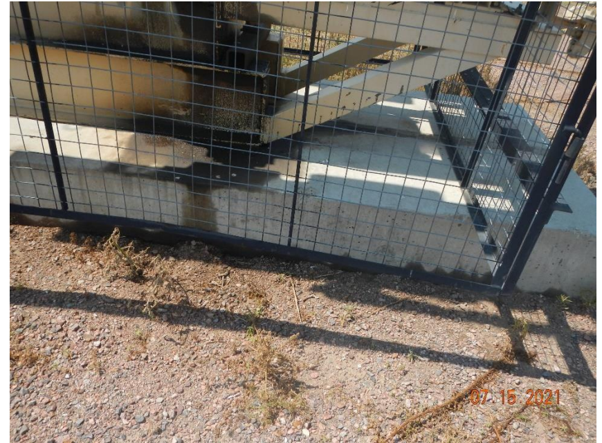
Gear box leak
