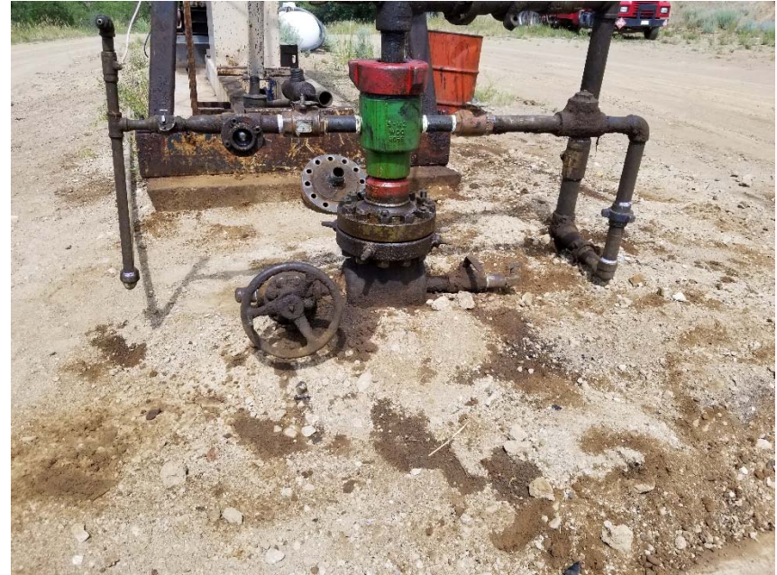
Photo 4. Stained soil at wellhead. No bradenhead access apparent.
