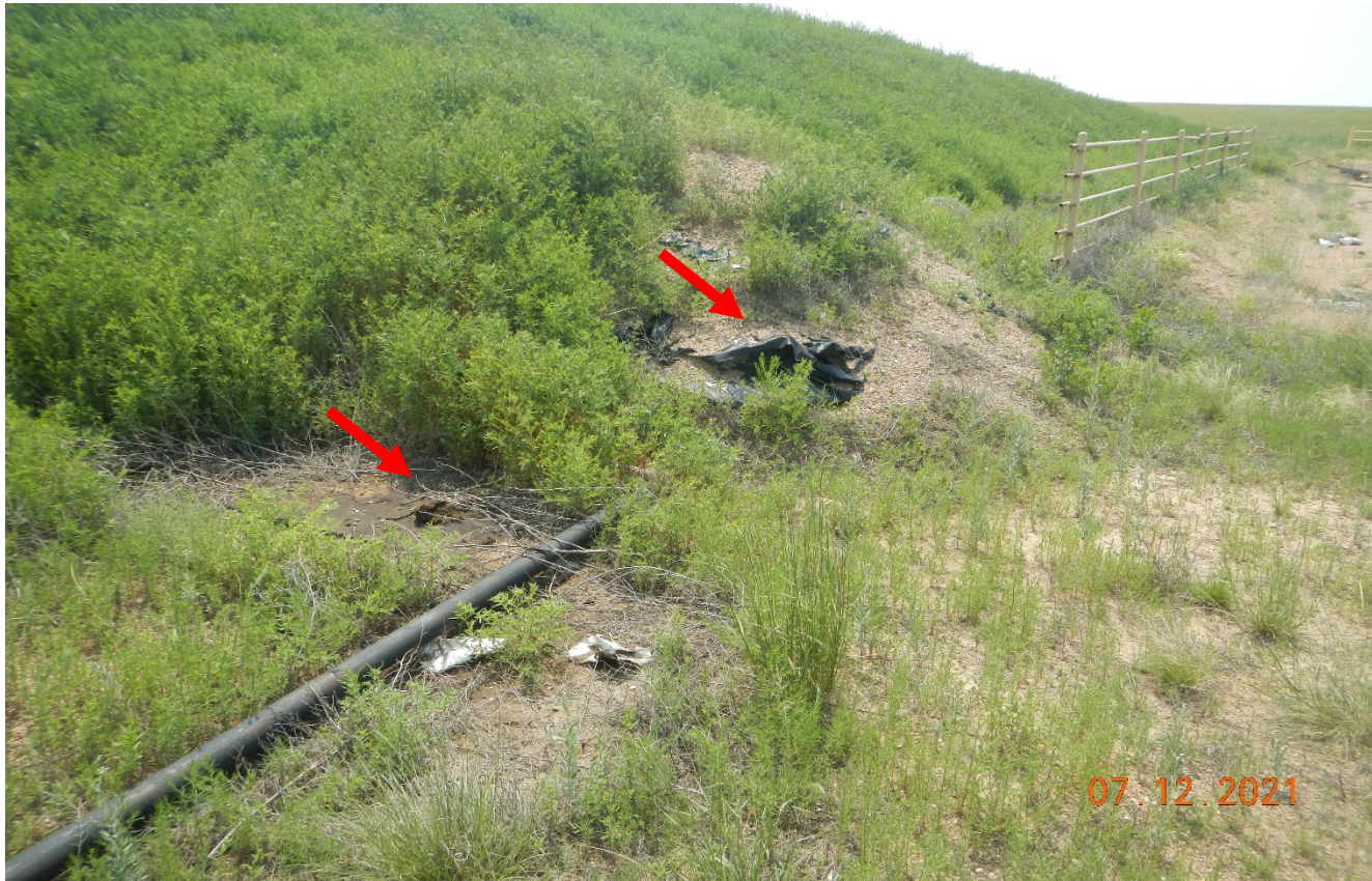
Photo 12. Facing southwest along the soil pile which is cover with undesirable weeds (Kochia). There is also a pile liner debris and oil stained soil shown at red arrow.
