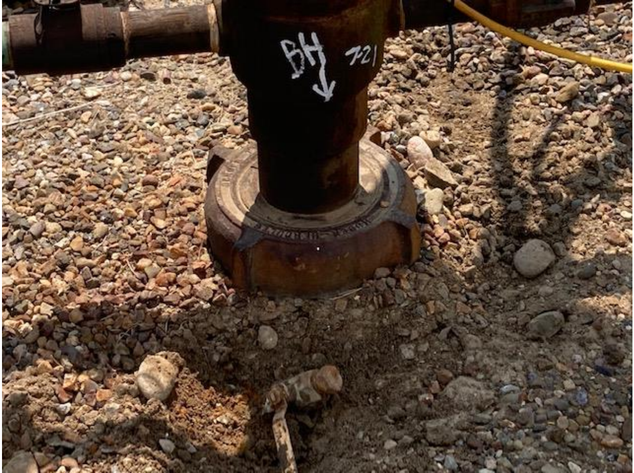
Bradenhead is plumbed to the surface to comply with Rule 341.
