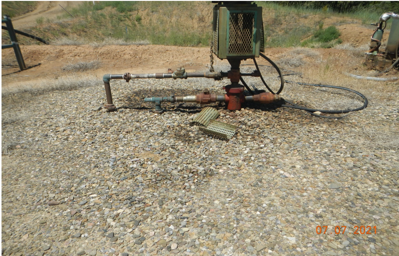
Photo 6. There is stained gravel around the wellhead indicating a previous leak.
