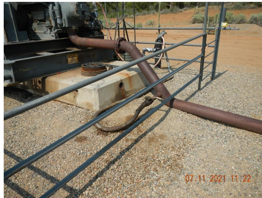
Stained gravel beneath prime mover exhaust.
