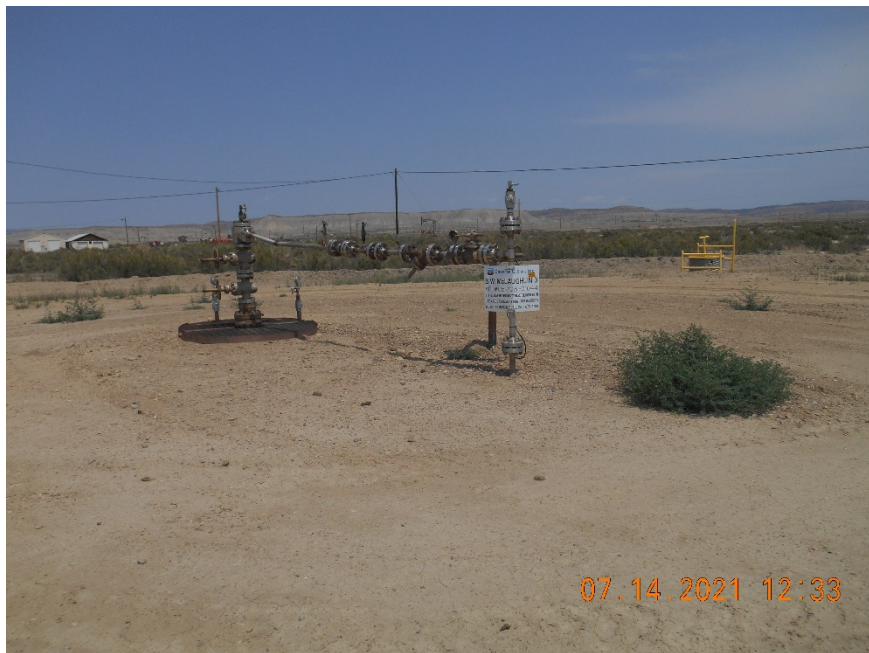
Injection wellhead.
