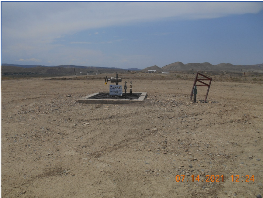
Injection wellhead. Temporarily Abandoned
