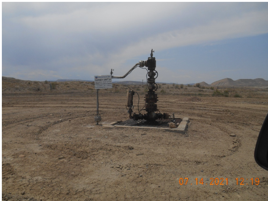
Injection wellhead
