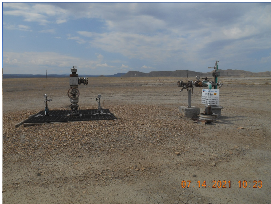
Injection wellhead. Temporarily Abandoned
