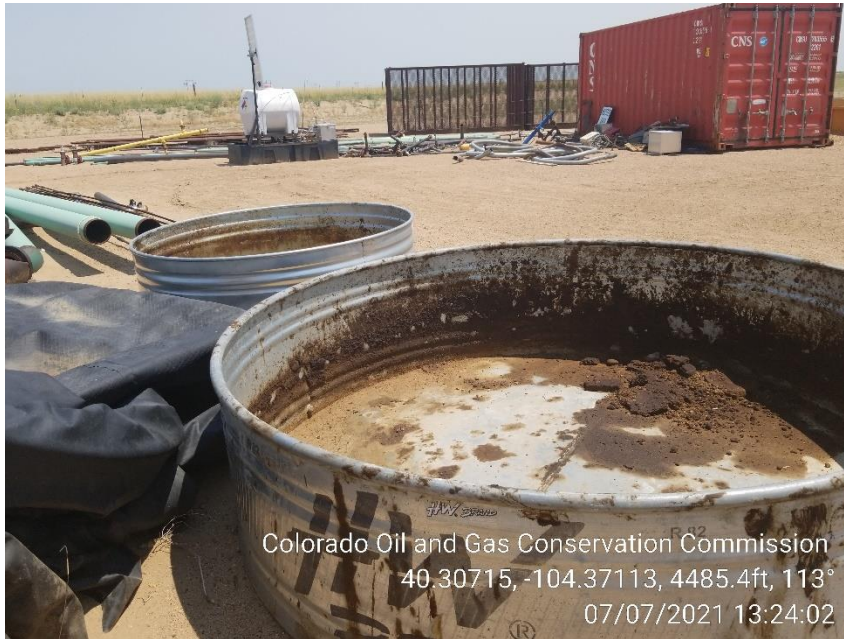
Photo 3 – Containment missing Wildlife netting
