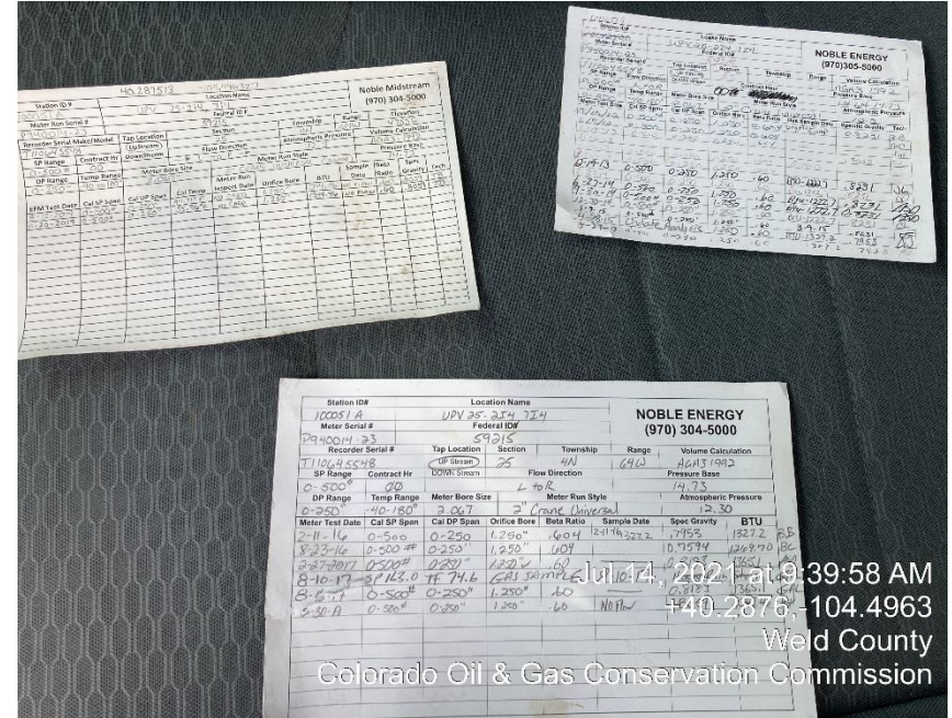
Photo #5 Meter not calibrated annually.
