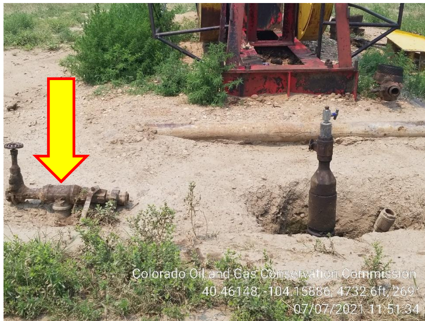
Photo 15 – Wellhead – Unmarked Riser – Weed Re-Growth
