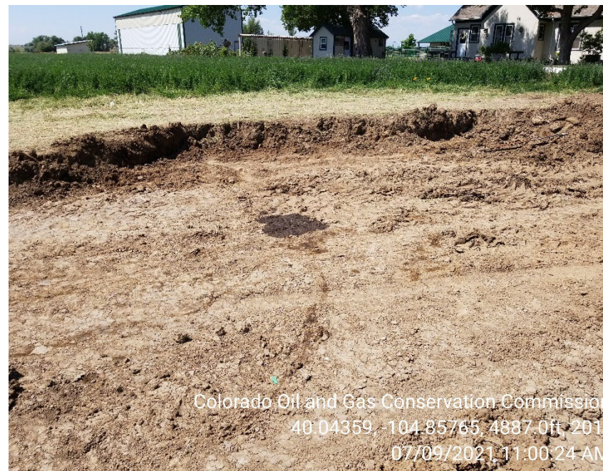
Photo 4 – Soil staining on surface in scraped area.
