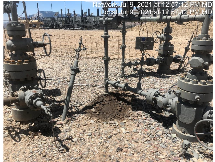
Photo #4377 Stained soils at wellheads.
