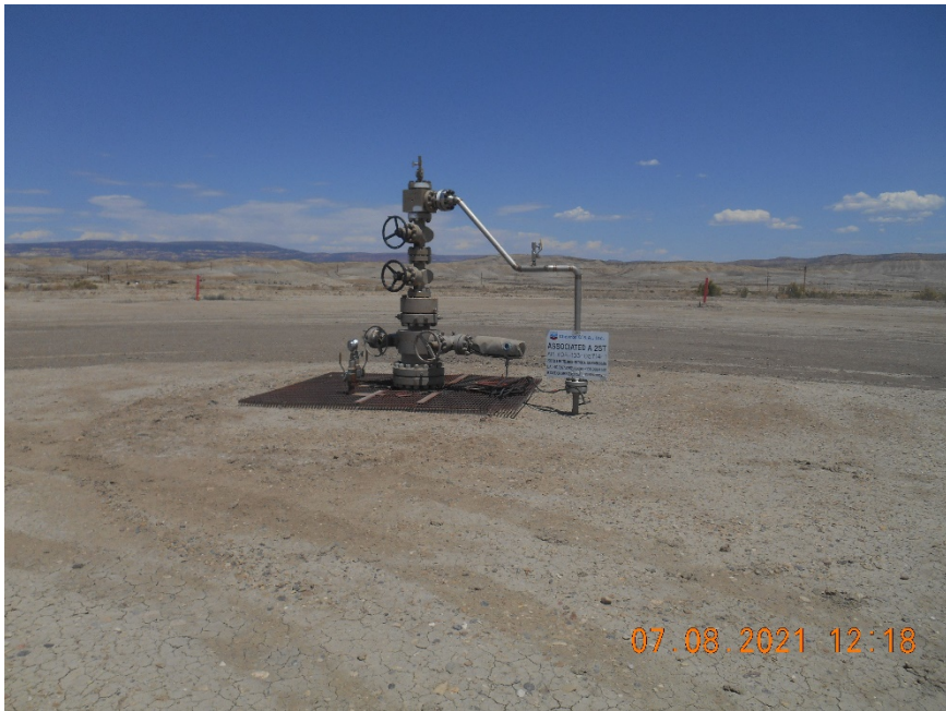
Injection wellhead.
