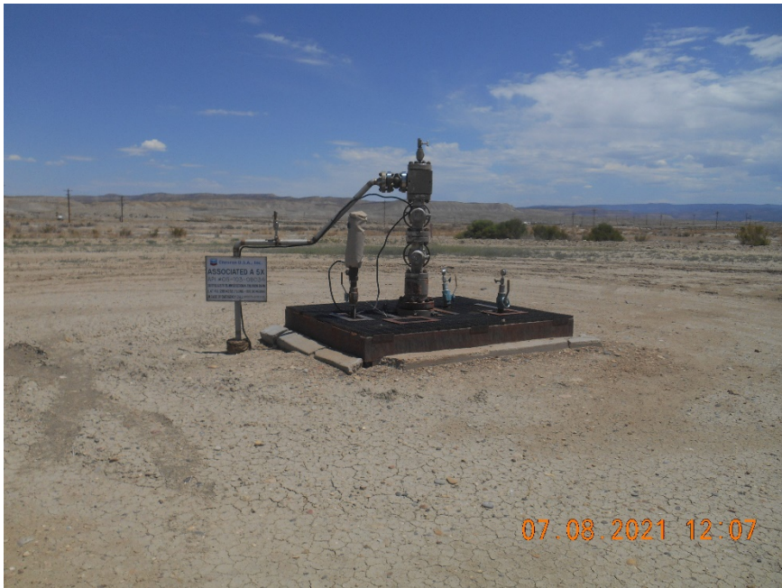
Injection wellhead.
