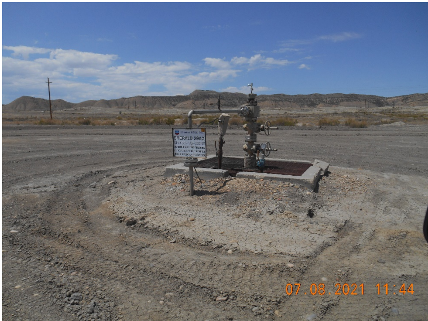
Injection wellhead
