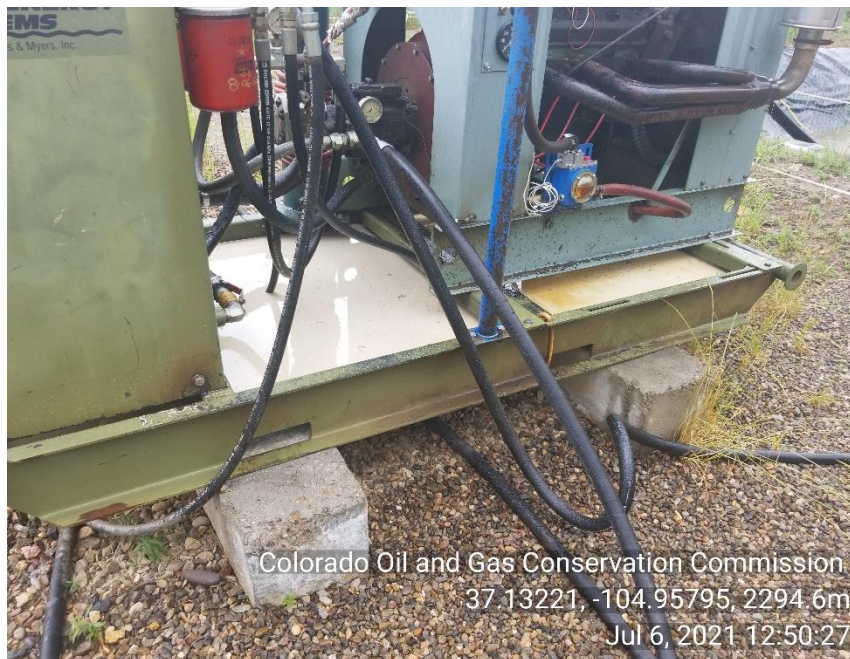
Photo 5 HYD motor skid full of fluid
