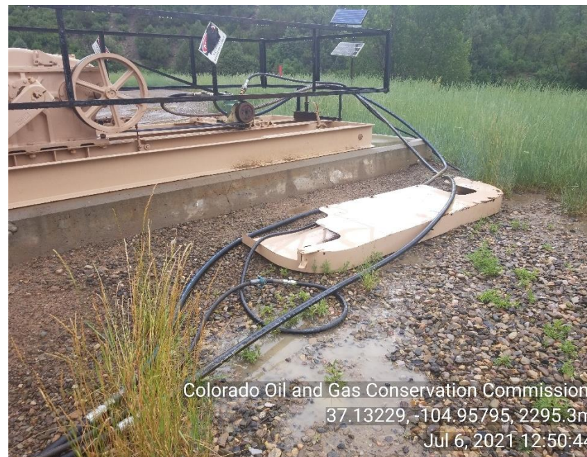
Photo 6 belt guard on ground.
