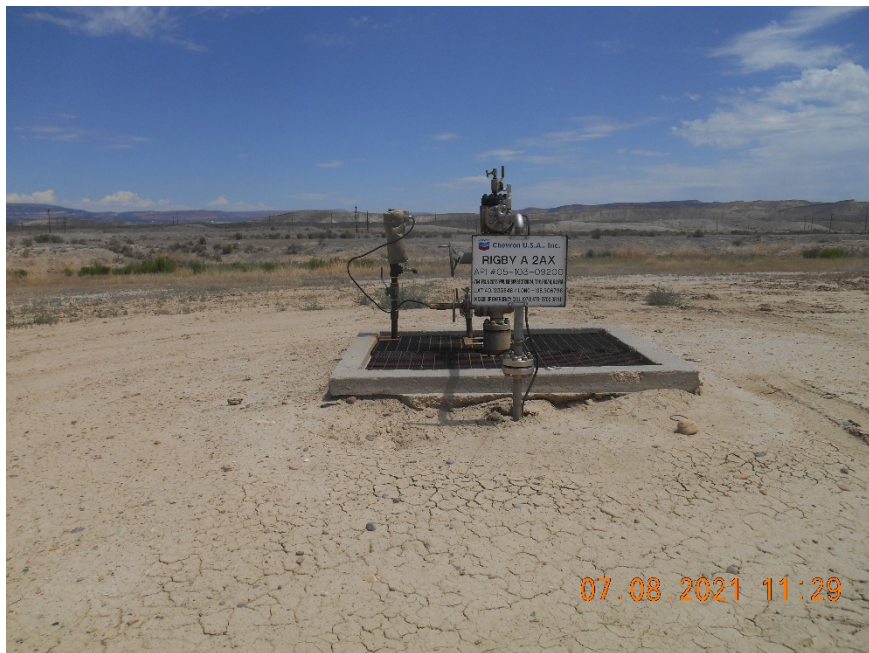
Injection wellhead
