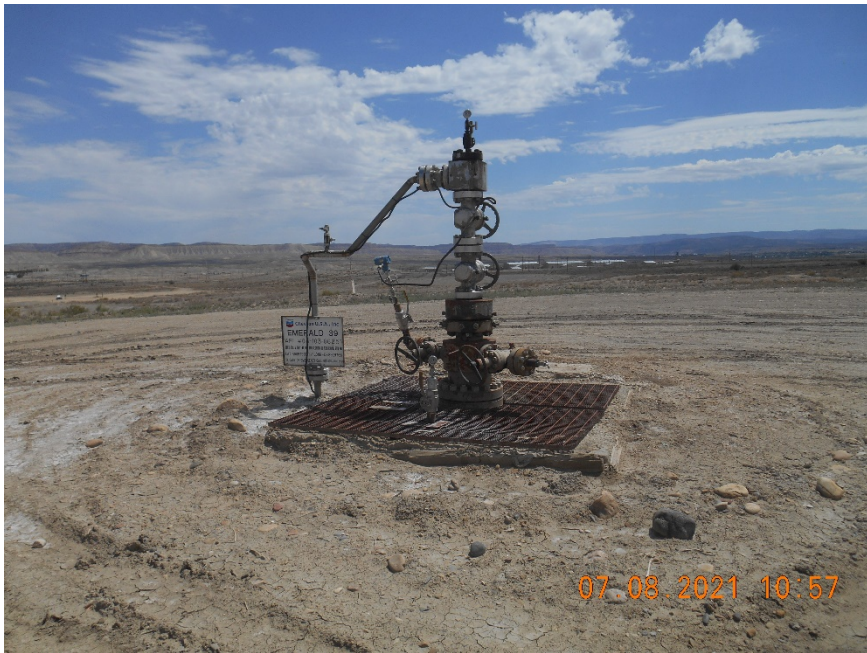
Injection wellhead.
