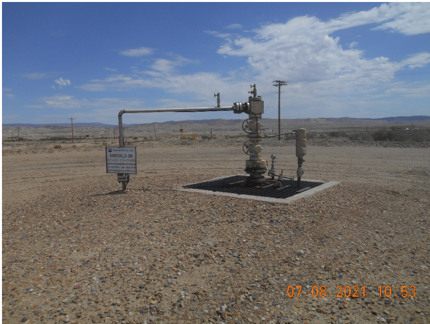
Injection wellhead.
