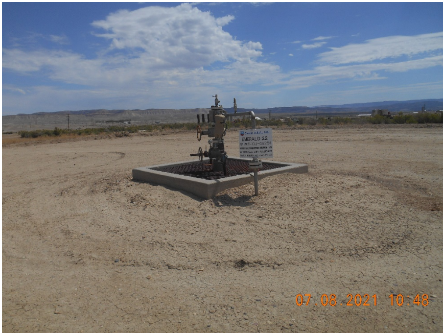
Injection wellhead.
